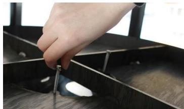
For easier assembly and disassembly, the screws must first be screwed into the main body.
