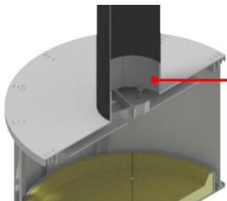
Self-tapping screws can be screwed in from the inside until the pipe is clamped. To access this spot, the deflector plate must be removed in advance.
