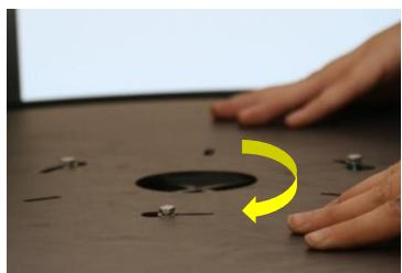
The plate can then be set on top, with the heads of the screws protruding through the enlarged holes in the slots. Then turn the plate and tighten the screws down in the narrowed end of the slots.
