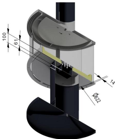
The 100 mm measurement is the distance between the underbody to the welded ring.
