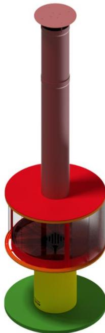
There is a risk of unintentionally touching hot parts when adding more wood. Open the glass panes as far as possible, to allow enough space to insert the piece of wood. Please take special note of the parts marked in red in the illustration on the left: there is a high risk to touch these parts unintentionally.
